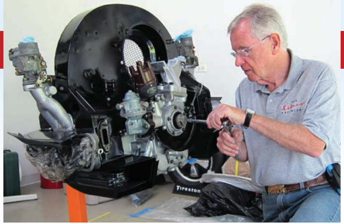
Finishing assembly of cleaned engine and painted sheet metal
