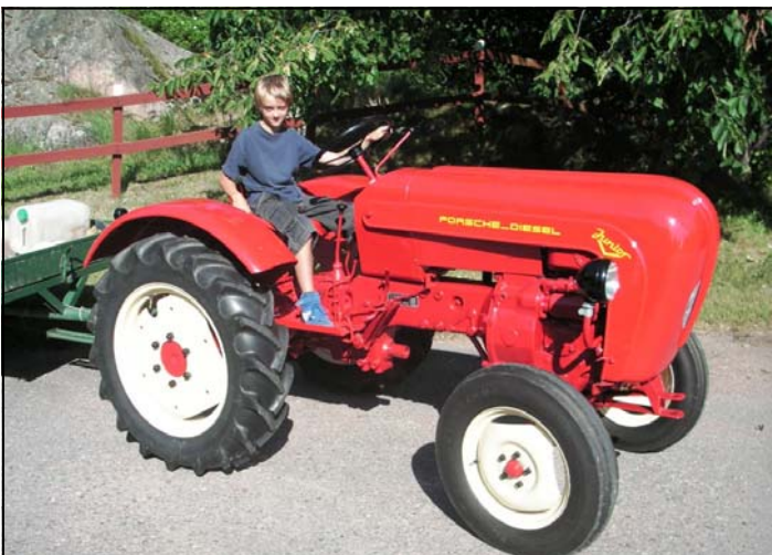
Porsche-Diesel Junior V from 1960 with son Johan in the driver seat. The tractor has a one cylinder air cooled (naturally!) diesel engine with 14 bhp.
