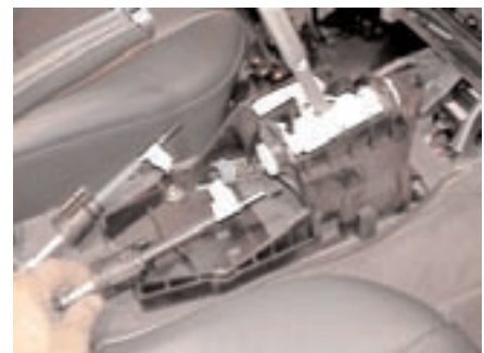
Photo C - Cables you should mark
