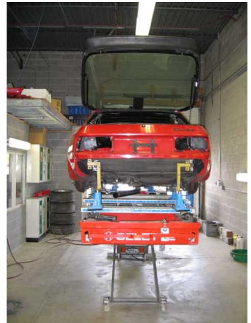
A bent 951S race car on the Celette Straightening Bench
