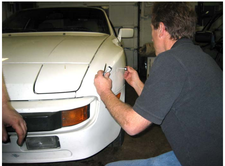
The dent magician puts the final touches on the 944. The dent repair was nearly invisible --- it would have likely been completely invisible, but Skiff quickly determined the presence of Bondo behind the original dent -the car had been damaged and repaired at least once before which caused some of the paint to fracture during this repair---which is being filled in here.
