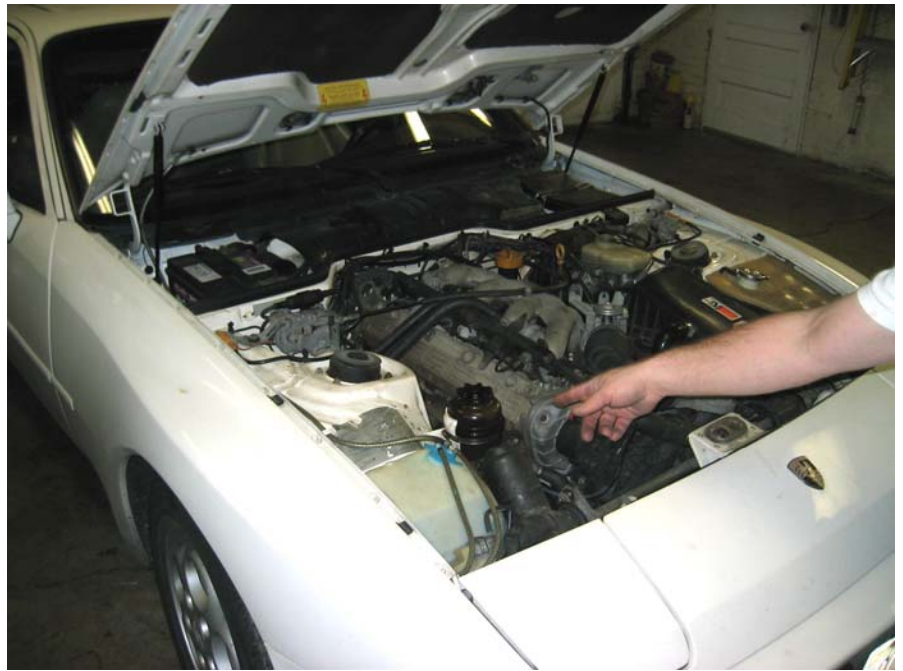
Karl points out the rubber shock tower caps that melted from the excessive engine heat.
