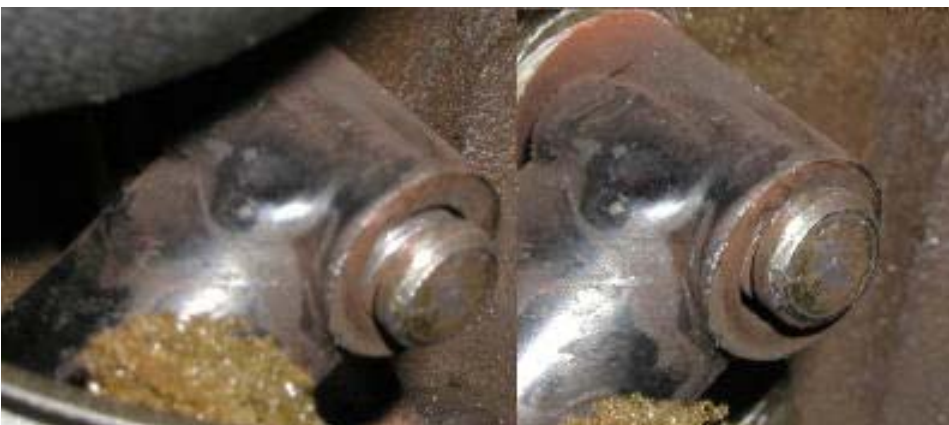
Note the excessive play in the shifter pin even after a new shifter is installed.
