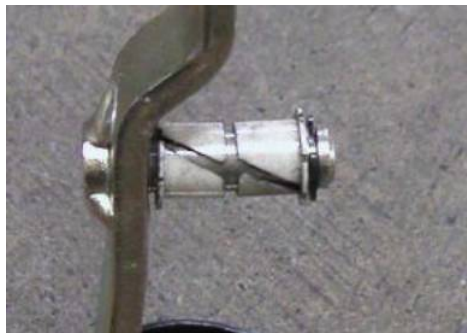
Where the old pivot pin was metal-to-metal we now have a Plastic bushing for smooth trouble free operation
