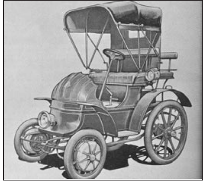
Porsche's 1899 Electromobile was unique in that it did away with a transmission by using electric motors mounted in the hubs of the front wheels, making it one of the first front-wheel drive-automobiles.
