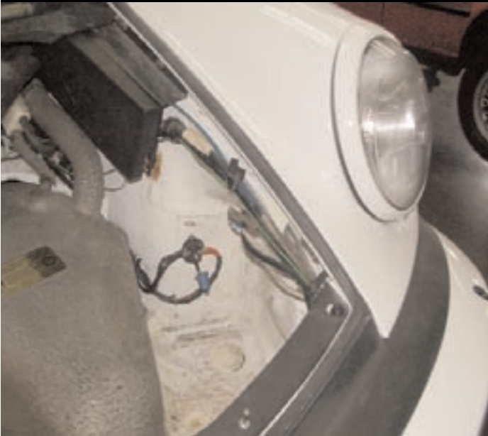
(Figure #3 – The 928 power junction neatly joins the 6-gage wire from the battery to the factory wiring harness allowing access for power, testing or charging)
