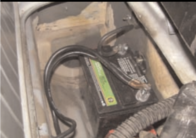
(Figure #4 - With the battery installed, we can see how well it fits with the cable routing, and battery tie-down clamp in place.
