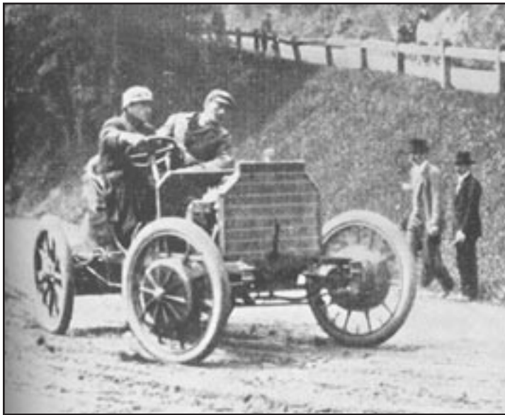
Ferdinand Porsche, shown here driving one of his Lohner-Porsche 'Mixte' cars in a hill climb, added a gasoline engine to replace the batteries and produce electricity for the motors built into the front wheels. His gas/electric hybrid was a winner almost 100 years before Toyota and Honda brought the hybrid automobile to market.
