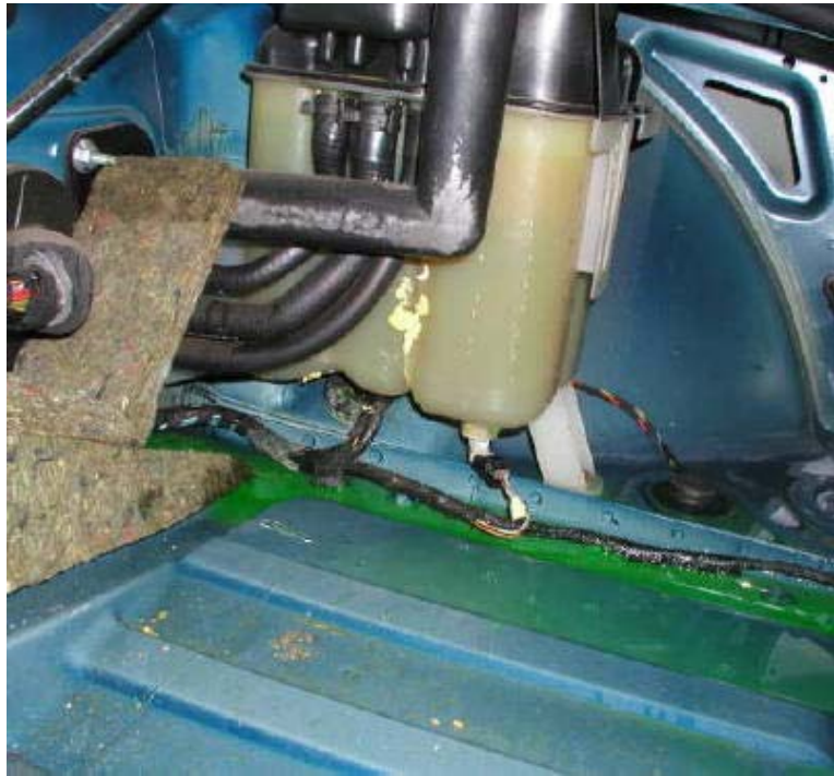
Figure #2: Notice the lake of coolant on the trunk floor and the coolant deposits on the side of the tank.
