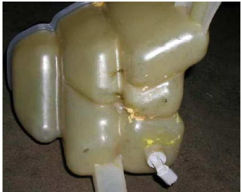
Figure #4: Hold tank up side down and look for discoloration at leak points.
