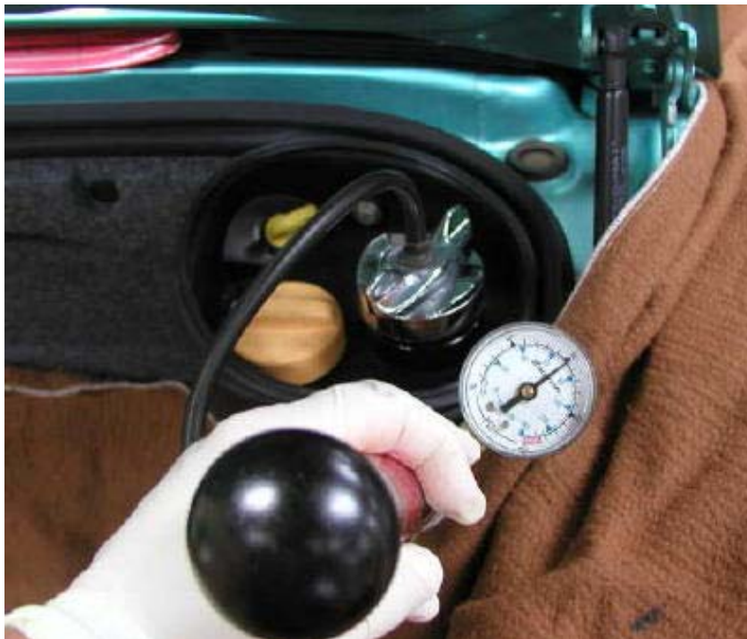
Figure #1: Coolant pressure tester and adapters are installed to replicate pressure under operating conditions
