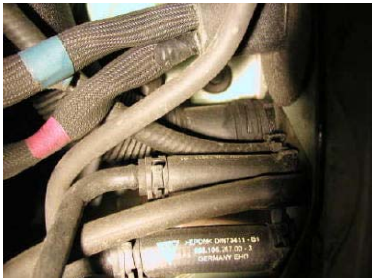
Figure #3: Fittings are way up into this cavity between the engine and trunk firewall. (This is a good time to find a small-handed helper)
