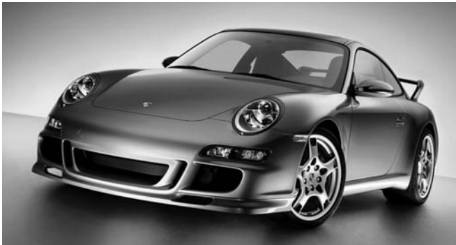
AEROKIT CUP FRONT APRON WITH LARGER INTAKES AND LIP SPOILER
