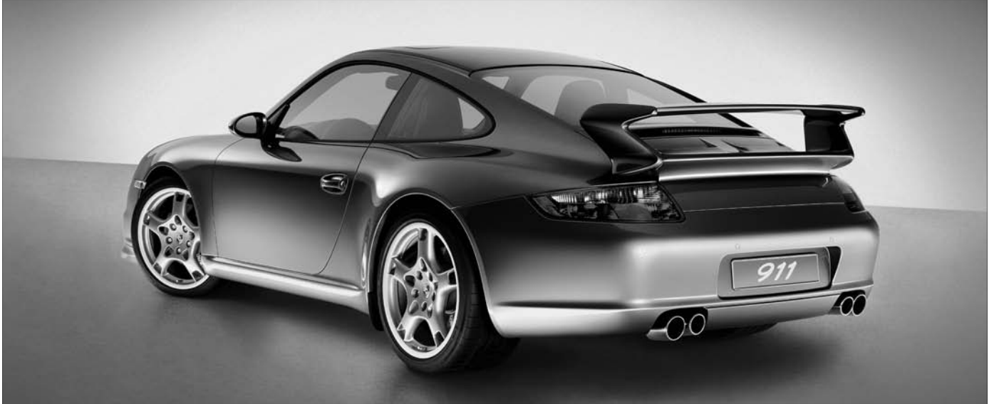
AEROKIT CUP WITH FIXED DOUBLE-WINGED REAR SPOILER
