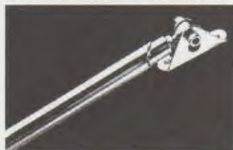
STRUT TOWER BRACES
