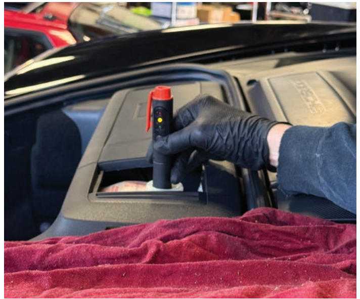
Hydroscopic test to determine if water has been absorbed into the brake fluid
