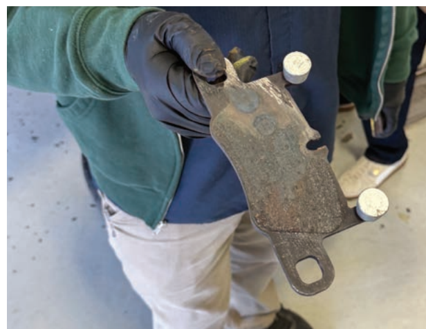
Brake pad is far past wear life. This could result in an expensive repair if driven on track.
